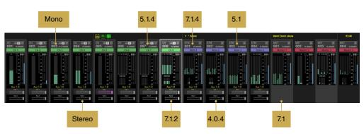
Channel View and S500 meterbridge path meters support all the path formats.
